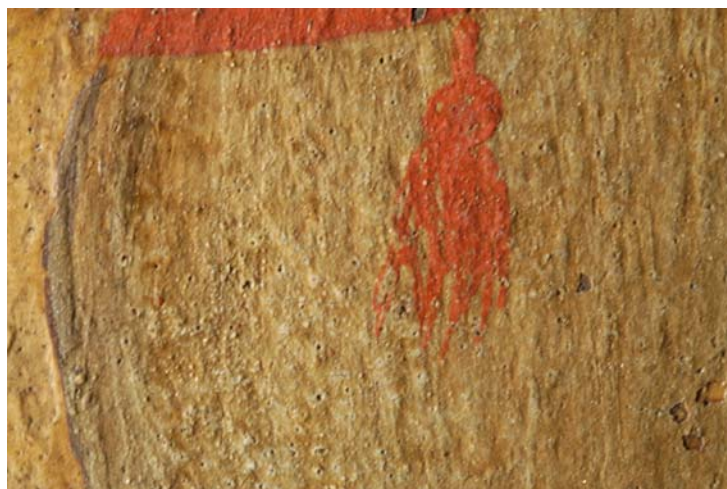
Fig. 3 – The icon of St. George, 17th century - Protrusions and crater-like voids due to the formation of lead soaps in the surface of a lead-white layer
