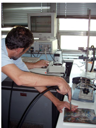
Figure 5a: Spot analysis of The Baptism with FT-NIR technique at NHRF.
