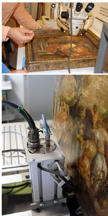
Figure 5b – 5c: Examination of The Adoration under the stereoscope, conservation dept. of the Benaki Museum; spot XRF analysis at NCSR Demokritos.
