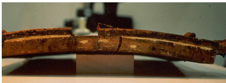
Figure 22 Detail of the central wing's upper section where we implanted wooden joints transversely to the cracks and inlaid balsa wood pieces in the gap between the wooden support and the frame's second level.
