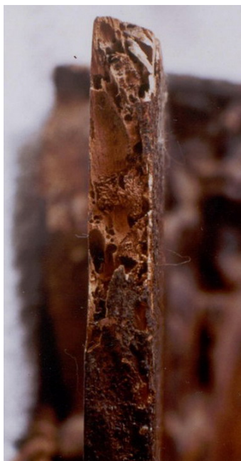
Figure 16 Detail from the upper left part of left wing's left section. The activity of wood destroying insects has cause losses of wood.
