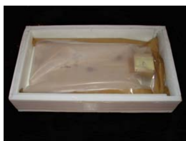
7. The second wood specimen along with a data logger, tape sealed in polyethylene plastic and placed in the polyurethane foam core box that is also tape-sealed, using thermic tape.
