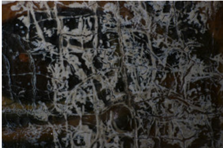
Figure 3: St. Nicolas. Photograph under stereomicroscope. The milky appearance of the crazing is more apparent in the edges of the cracks.
