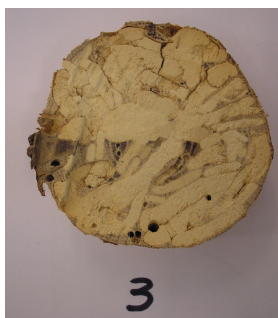
Picture 30: Cross section of the sample after consolidation.
