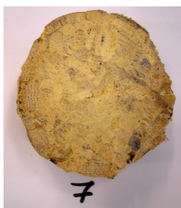
Picture 50: Cross section of the sample after consolidation.
