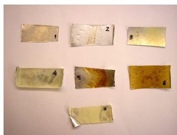
Picture 18: Polymers sample films, after heating ageing test.
