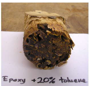
Picture 49: 7th sample after consolidation.
