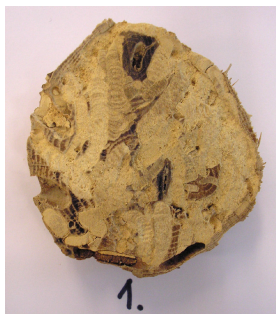
Picture 20: Cross section of the sample after consolidation.
