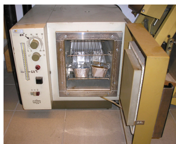
Picture 17: Samples in the oven, during the heat ageing test.
