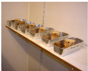
Picture 6: Samples during consolidation
