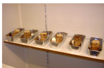
Picture 7: Samples after the first hour of consolidation treatment.
