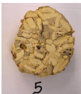
Picture 40: Cross section of the sample after consolidation.
