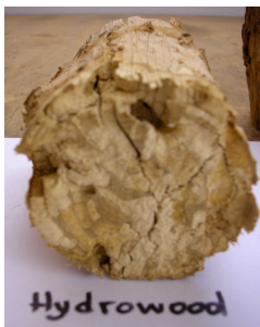
Picture 44: 6th sample after consolidation.
