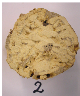
Picture 25: Cross section of the sample after consolidation.
