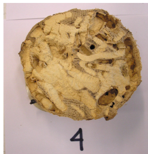
Picture 35: Cross section of the sample after consolidation.
