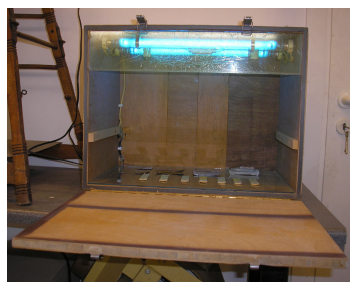
Picture 15: Close box with Ultra Violet light source.
