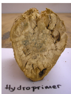
Picture 39: 5th sample after consolidation.
