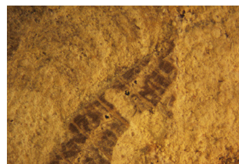
Picture 21: Photo of wood's texture through the optical microscope 10X magnification.
