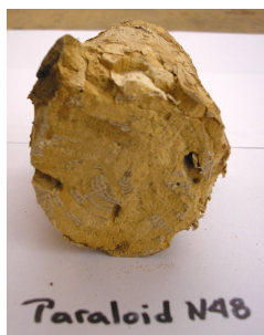
Picture 29: 3rd sample after consolidation.
