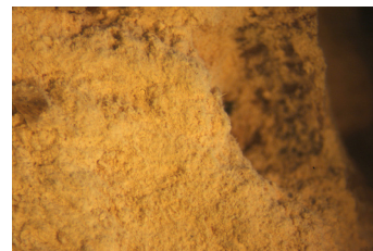
Picture 36: Photo of wood's texture through the optical microscope 10X magnification.
